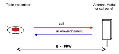
The call of the table transmitter is received by the Antenna module which immediately is sending back an acknowledgement to the table transmitter. (If this is not received, the table transmitter automatically is re-dialling once or twice)
