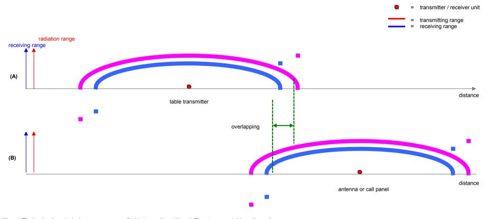
(A) and (B) showing the principal coverage ranges of table transmitters (A) and (B) antenna modul (or call panel).
