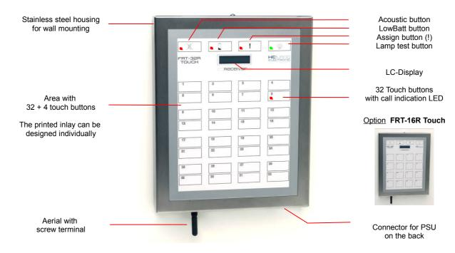
The FRT-32R-Touch is a wireless Call Indication Panel for up to 32 call buttons (table transmitters et al.). The slim and easy to clean stainless steel housing can be fixed to the wall by 2 screws like a picture. Incoming calls from up to 32 call buttons are indicated at the respectively assigned buttons and the LCD is showing all calls in order of its reception.
