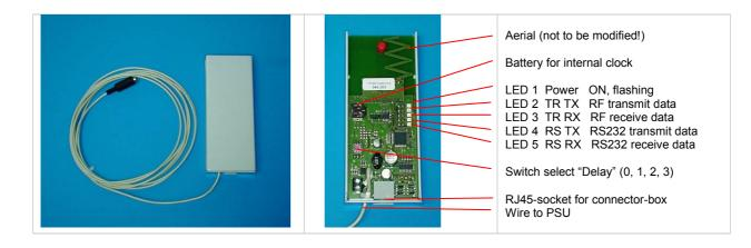
The Repeater is used to extend the range of RF transmission between the transmitters (call buttons, call panels etc.) and receivers (indication panels, pagers). For best performance the repeater is positioned as high as possible above ground and away from metal surfaces. It is supplied by a plug-on power supply unit. This repeater also contains an internal clock to allow transmission of the actual time to the display of the Mini-Pagers.
