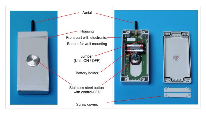
The Call Button FRT-WS 1 is used for manual operation in industrial locations to call for assistance or requesting supply of material . The call can be received at one or more mobile or stationary receiver units with visual and / or acoustical announcement or transfer the call button's ID-code via a serial RS-232 interface to a connected PC or similar for further processing.
