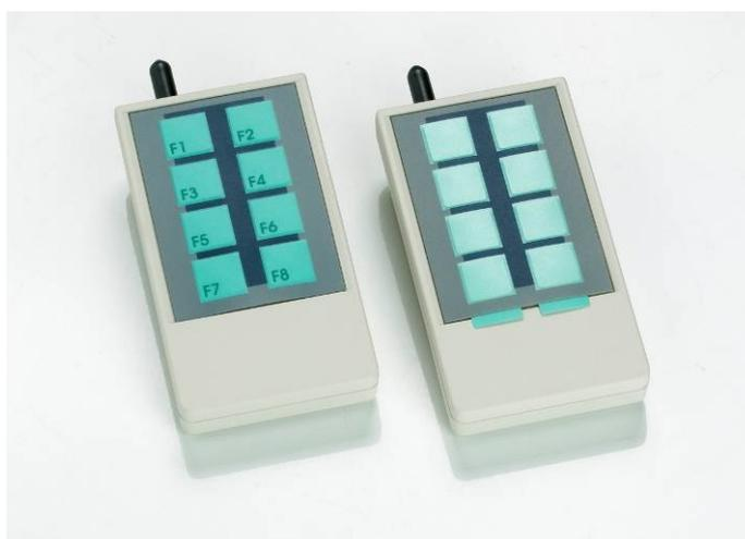
The 8-button transmitter FRT-HS 8 is a handheld unit for RF transmission of up to 8 commands, which can be received and indicated visually and/or by tone or which can switch up to 8 relays. The 8 buttons can either be imprinted with „F1“ ... „F8“ or can be blank, having two detachable strips for an individual inscription.
