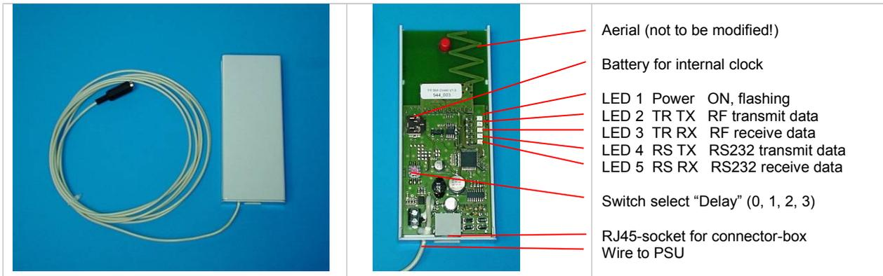
The Repeater is used to extend the range of RF transmission between the transmitters (call buttons, call panels etc.) and receivers (indication panels, pagers). For best performance the repeater is positioned as high as possible above ground and away from metal surfaces. It is supplied by a plug-on power supply unit. This repeater also contains an internal clock to allow transmission of the actual time to the display of the Mini-Pagers.
