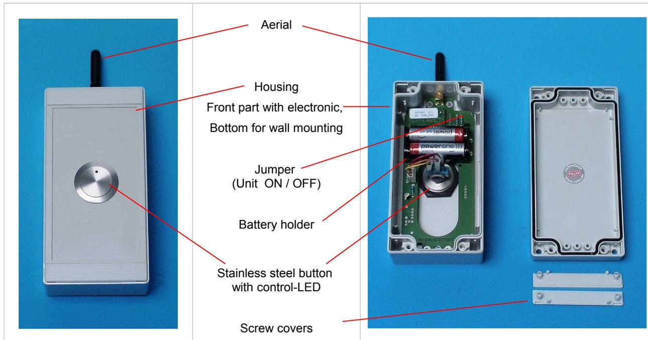
The Call Button FRT-WS 1 is used for manual operation in industrial locations to call for assistance or requesting supply of material. The call can be received at one or more mobile or stationary receiver units with visual and / or acoustical announcement or transfer the call button's ID-code via a serial RS-232 interface to a connected PC or similar for further processing.
