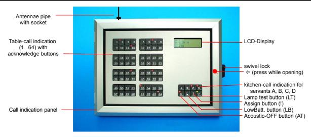
The FRT-32 (-64) LCD is a wireless Call Indication Panel for up to 32 (64) Call Buttons (table transmitters et al.). The slim alloy housing can be fixed to the wall by 2 screws like a picture. Incoming calls are indicated at the respectively assigned buttons and the LCD is showing all calls in order of its reception.
